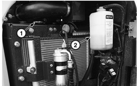
Coolant Recovery Tank
