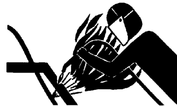
Heating Near Pressurized Fluid Lines
